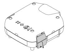
Loosen the two screws securing the lamp housing until the screwdriver goes into a freewheeling condition. Remove the lamp housing by pulling it out by the handle.
