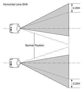
If the lens is shifted both horizontally and vertically, the maximum range in either direction is reduced due to the rounded off area near the edge of the lens (see below).
