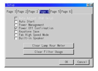
**Auto Adjust (RGB Only)** - When checked, the projector automatically determines the best resolution for the current RGB input signal. The projector can automatically adjust the Horizontal and Vertical Position along with Clock, Phase and Resolution.
