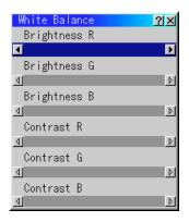
To make adjustments use the up and down cursors to select the item to modify then use the left and right cursors to make the adjustment.
