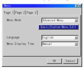
2. Use the up and down cursors to highlight your selection and press the Enter button to place a check mark next to an option to enable that feature in the menu system. Pressing the Enter button over a checked box will deselect it. If you select an item with a solid triangle to the right of it and press Enter, you will enable all sub menu items under that feature.
