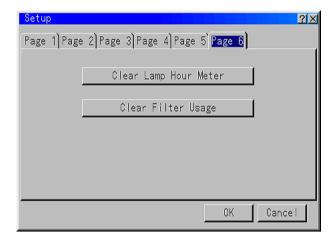
**Clear Lamp Hour Meter** - Resets the lamp clock to zero. Selecting this option displays a confirmation window: To reset the lamp usage hour, press 'OK'.
