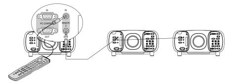
Next, assign a unique ID number to each projector and operate using the remote control as normal. The ID number can be set to 'None' allowing multiple projector control (see operation via remote control on previous page).
