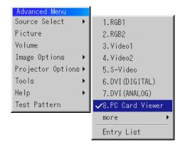
Checking 'Show Folder List' means that selecting PC Card Viewer input displays a list of all folders in the PC Card and if 'Auto Play' is checked the projector automatically starts to play slides at the first slide of the folder you have selected.
