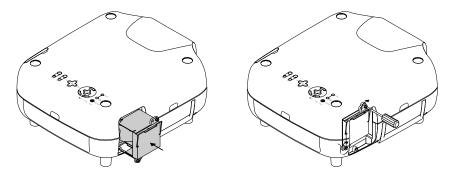
Attach the lamp cover and secure by tightening the attached screw.
