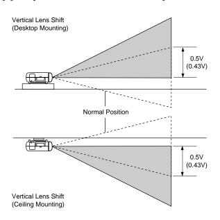
As with vertical positioning, the default horizontal position of the projector is at the centre of the screen. However, the projector can be mounted to the left or right of image centre and the 'Lens Shift' function used to centre the image on screen. The maximum horizontal lens shift range is 25% of the projected image width.
