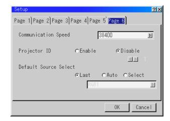
**Communication Speed** - Defines the baud rate of the PC CONTROL connector.
