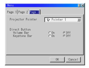
**Projector Pointer** - This option is available on the optional presentation remote control (PR50KIT) only and enables you to select from eight different pointer icons for the 'Pointer' button on your remote control.
