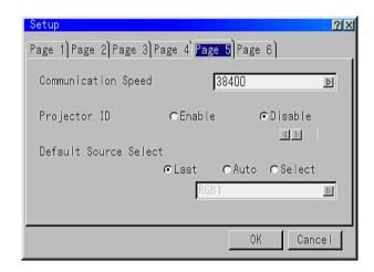
**Communication Speed** - Defines the baud rate of the PC CONTROL connector.
