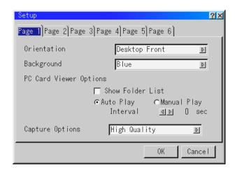
**Orientation** - The projector can be set for desktop front projection, ceiling rear projection, desktop rear projection or ceiling front projection.
