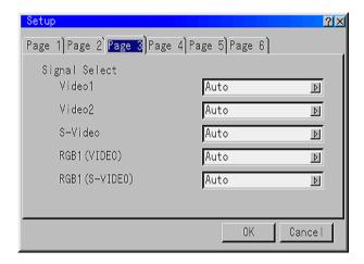
**Signal Select** - Allows you to define the type of RGB and VIDEO input signals.
