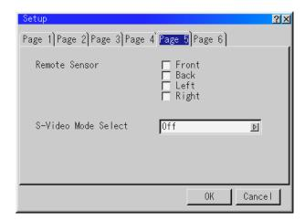
**Remote Sensor** - Determines which infra red sensors are enabled for remote control operation.
