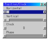
Horizontal and vertical position allows you to manually adjust the position of the displayed image on the screen using the left and right cursor buttons.
