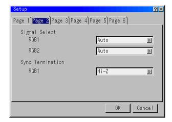
**Signal Select** - Defines the input signal type for the RGB 1 and RGB 2 inputs. The options are 'RGB', 'Component' and 'Auto'. Normally 'Auto' would be selected to allow the projector to automatically select the input type. However, there may be certain signal types that the projector is unable to detect. If this is the case, 'RGB' or 'Component' can be defined.
