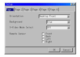
**Orientation** - The projector can be set for desktop front projection, ceiling rear projection, desktop rear projection or ceiling front projection.
